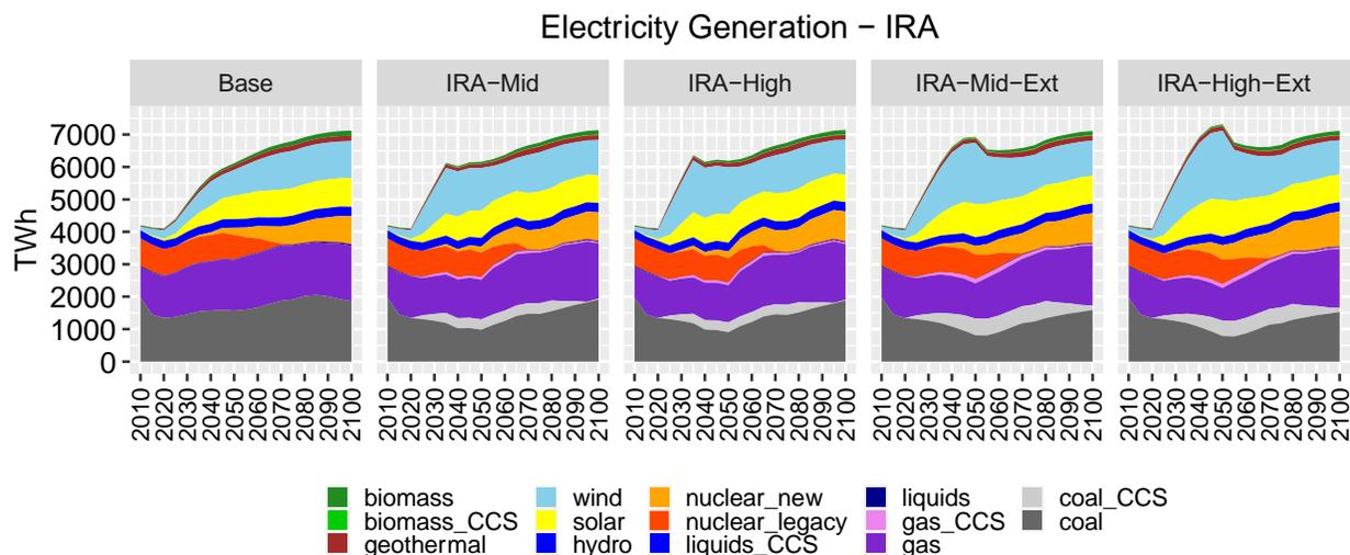
Figure 23. Electricity generation by fuel for alternative IRA scenarios (TWh).
