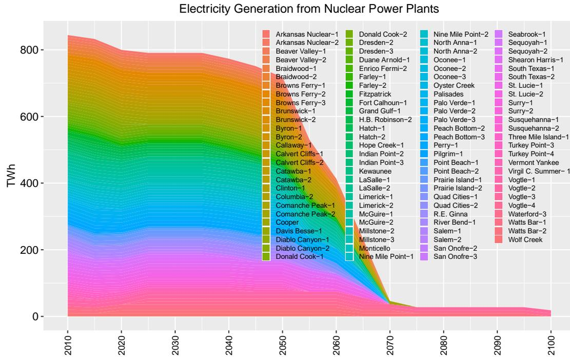
Figure 1. Electricity generation from existing nuclear power reactors in the US assuming 80-year lifetimes, except for Diablo Canyon 1&2, and including Watts Bar-2, Vogtle-3, and Vogtle-4 reactors.
