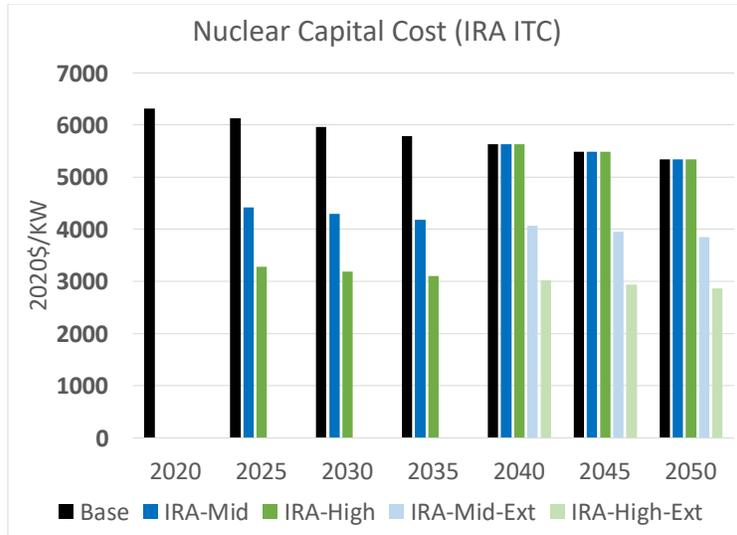
Figure 4. Nuclear reactor capital costs for Base case and adjusted costs for alternative IRA cases.
