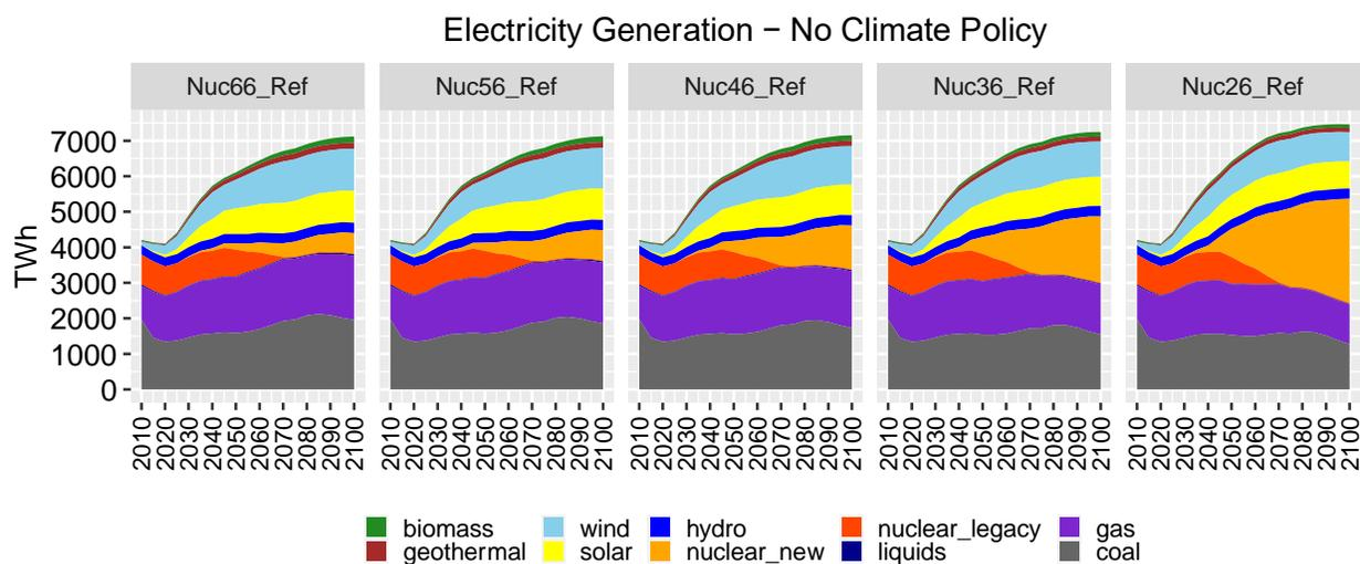
Figure 16. Electricity generation by fuel type in Reference scenario for alternative nuclear capital cost cases (TWh).
