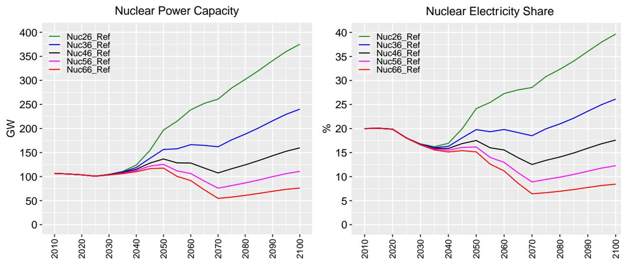
Figure 17. Nuclear power capacity and share of electricity generation in Reference scenario for alternative nuclear capital cost cases.
