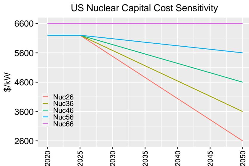
Figure 2. Nuclear power reactor overnight capital cost cases for the US at 2600, 3600, 4600, 5600, and 6600 \$/kW by 2050 (2020 USD).
