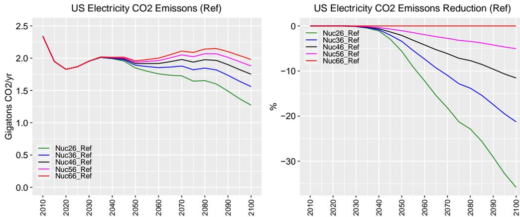
Figure 19. US electricity sector CO<sub>2</sub> emissions and impact of nuclear power capital cost reductions in the Reference scenario.
