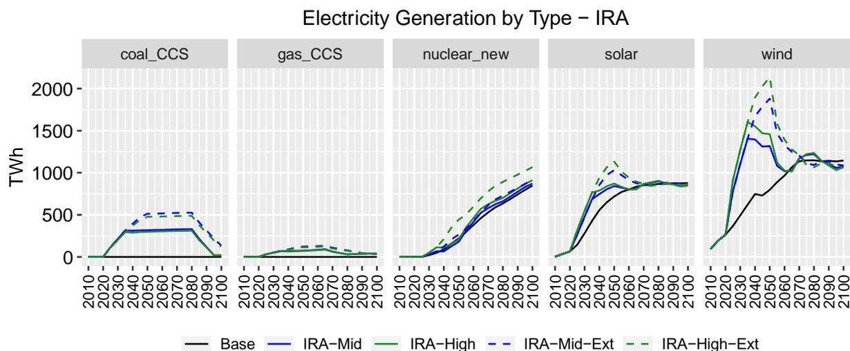
Figure 24. Comparison of electricity generation impact of IRA scenarios for clean power technologies (TWh).
