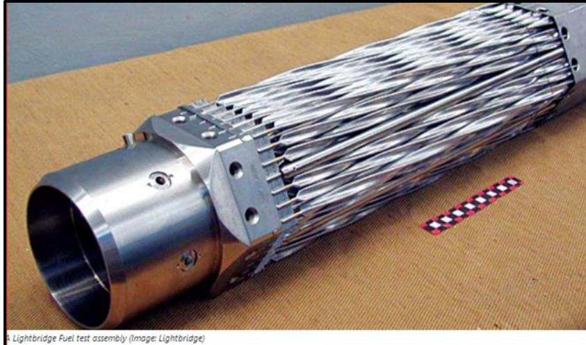
Figure D1-6A.8. A prototype Lightbridge/EnFission fuel assembly.
