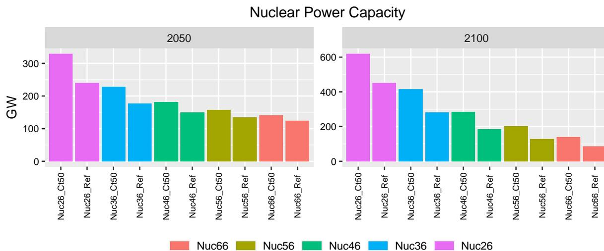
Figure 14. Comparison of nuclear power capacity in 2050 and 2100 for the Reference and 50 \$/tCO<sub>2</sub> carbon tax scenarios at alternative nuclear capital costs.
