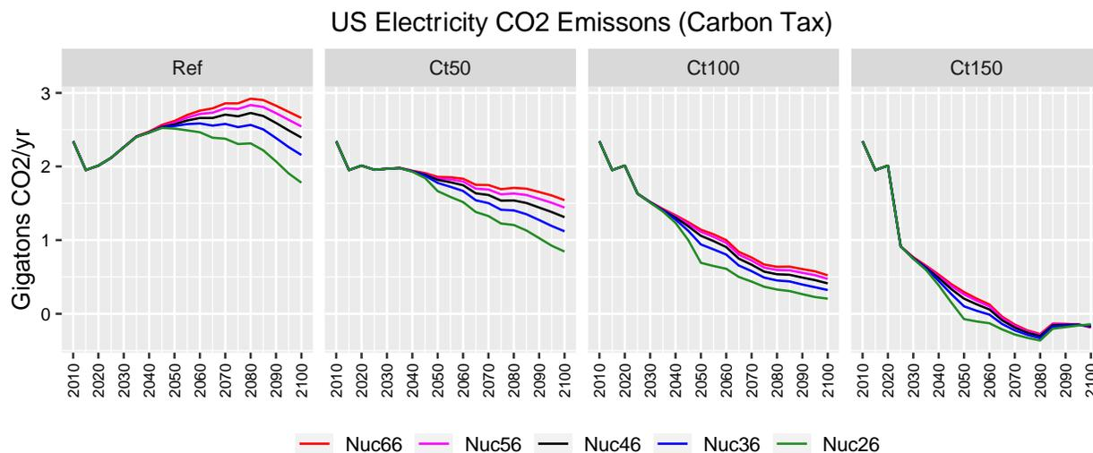
Figure 17. US CO<sub>2</sub> emissions from electricity generation for the carbon tax scenarios with alternative nuclear cost cases.
