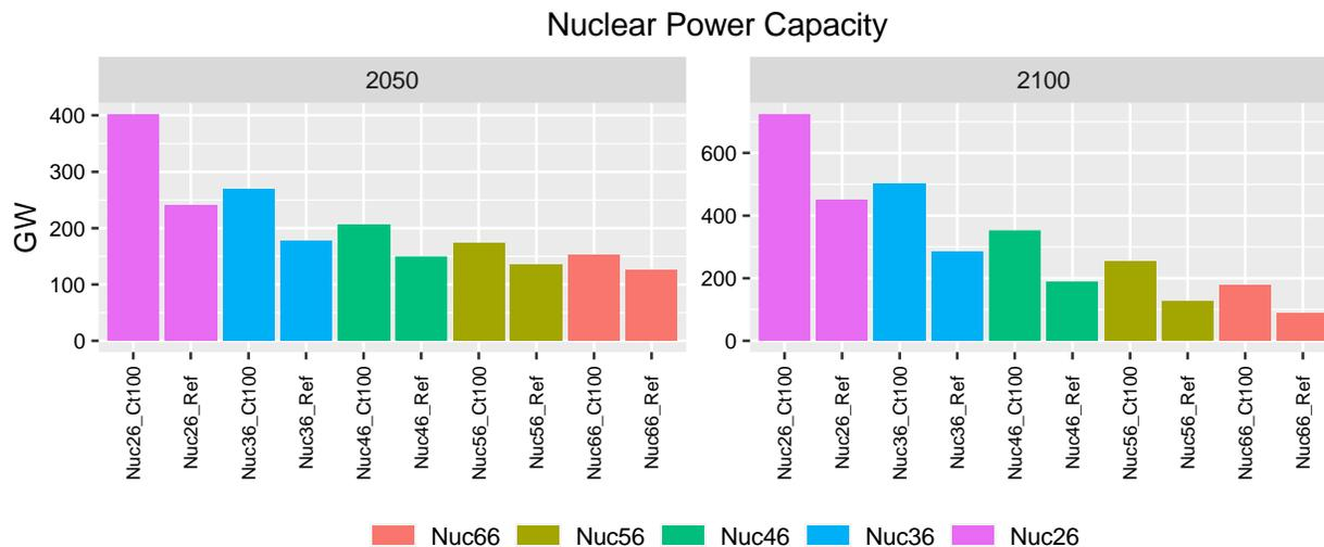
Figure 15. Comparison of nuclear power capacity in 2050 and 2100 for the Reference and 100 \$/tCO<sub>2</sub> carbon tax scenarios at alternative nuclear capital costs.
