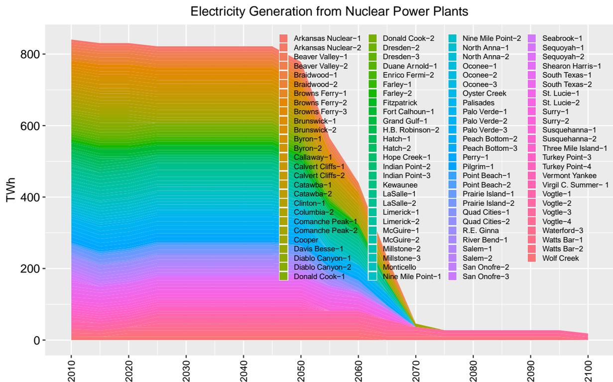
Figure 1. Electricity generation from existing nuclear power reactors in the US assuming 80-year lifetimes and including Watts Bar-2, Vogtle-3, and Vogtle-4 reactors.
