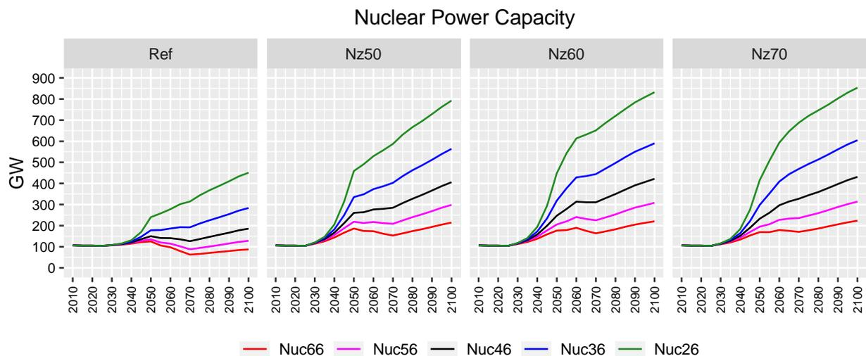
Figure 21. Nuclear power capacity in the net-zero emission scenarios for alternative nuclear cost cases.
