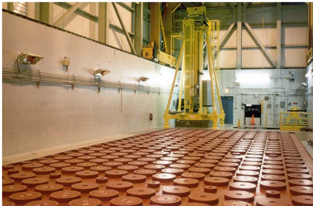
Figure E4-5. Fort St. Vrain modular vault dry store (MVDS) showing charge face.
