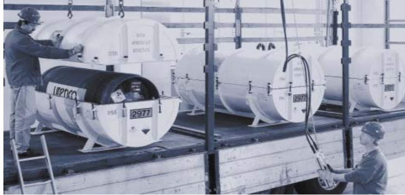
Figure C1–11 Enriched UF 6 product container being loaded into an overpack for shipment.
