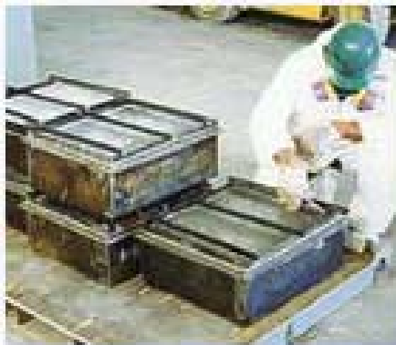
Figure G3-3. EnergySolutions microencapsulation and macroencapsulation of waste in plastic polymer. Figure taken from EnergySolutions Web site.
