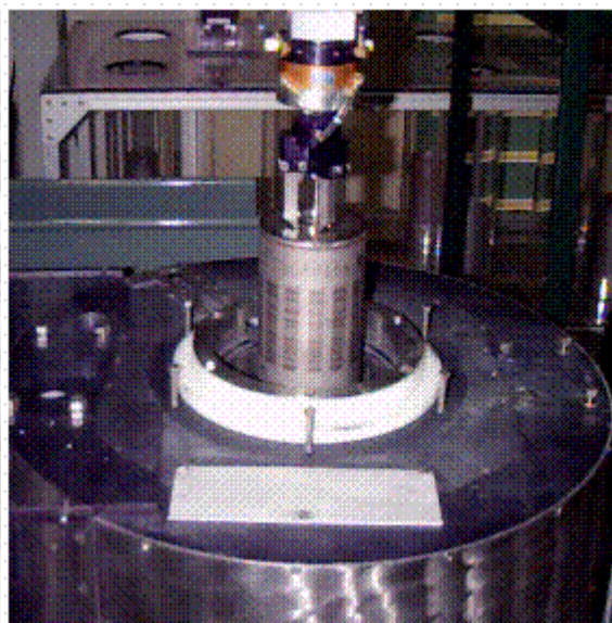
Figure 2. Crane Loading ITSC into Neutron Counter
