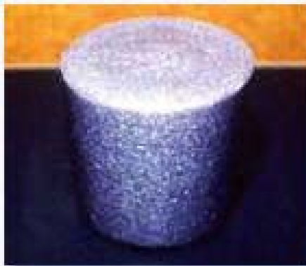
Figure G3-3. EnergySolutions microencapsulation and macroencapsulation of waste in plastic polymer. Figure taken from EnergySolutions Web site.
